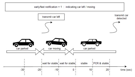
It is not possible to detect that the car has only moved and that the same car is in the same spot. In case of a bumper-to-bumper move where there is only a couple of seconds delay between an empty parking space and a newly parked car, we have the possibility to send a 'car left' message from the moment the car starts moving. It is not distinguishable if after this car had moved the same car is parker or another car is present.
