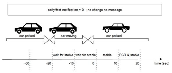
For guiding cars to a free parking space, it is of no use to transmit that the spot was free for a couple of seconds. Battery power can be retained by not sending a message. In the above scenario, a "quick" car change may not lead to signalling indications.
